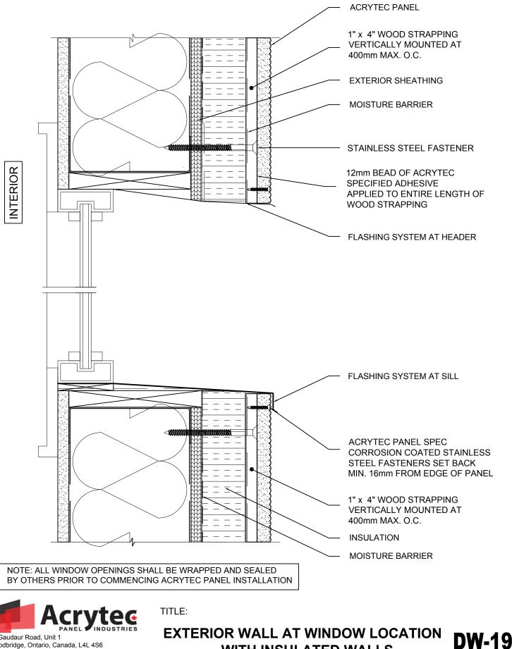
40 Gaudaur Road, Unit 1 Woodbridge, Ontario, Canada, L4L 4S6 T: 905.326.3749 I F: 905.326.2732 Toll: 1.800.316.9430 I www.acrytecpanel.com **EXTERIOR WALL AT WINDOW LOCATION** WITH INSULATED WALLS
