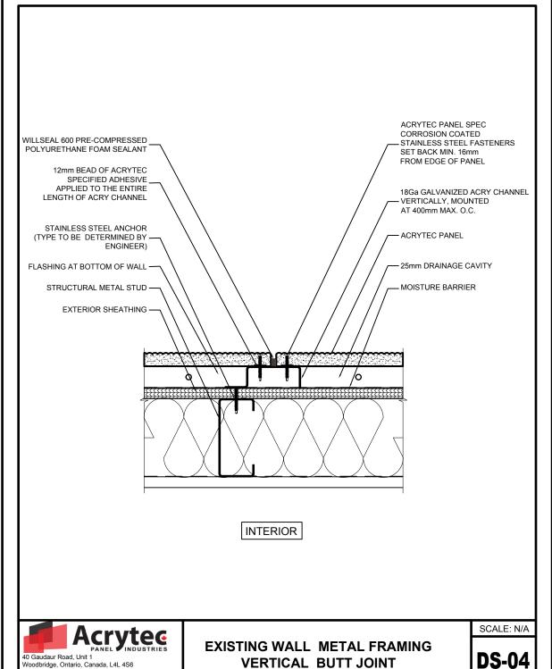
T: 905.326.3749 I F: 905.326.2732 Toll: 1.800.316.9430 I www.acrytecpanel.com **VERTICAL BUTT JOINT**
